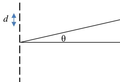
The grating constant is the reciprocal of the line spacing  $d$ . [# lines / length]
