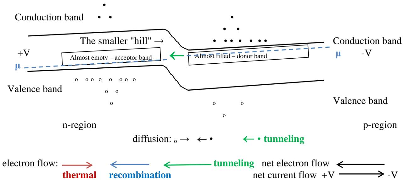
As the voltage is increased further, we get this situation: the p-side is slightly lower than it was, the n-side is slightly higher than it was; net effect is to reduce tunneling while increasing diffusion. The reduction in tunneling is greater than the increase in diffusion so the current goes DOWN with increasing voltage!
