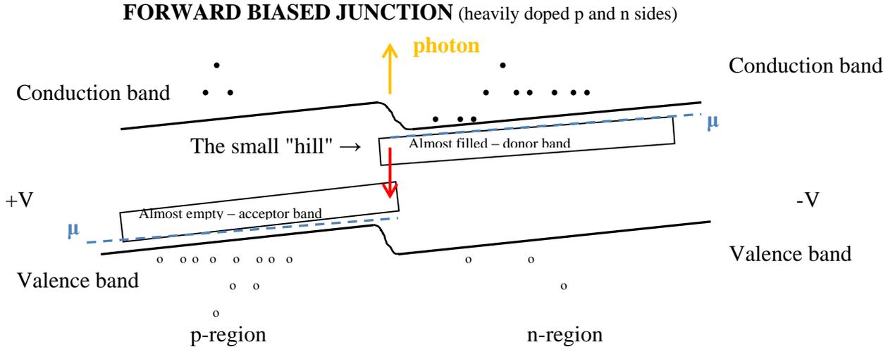
Recall that the energy given off by the electrons in falling into the holes will be **photons of energy equal to the energy gap**. Thus for visible light emitting diodes, we must make sure that the energy gap is at least that at the red end of the visible spectrum (as calculated on the previous page):  $E_{\text{gap}} > 1.78 \text{ eV}$ . This will then provide a low power way of providing light (of one color). Also note that we need a **direct gap** semiconductor for an LED.
