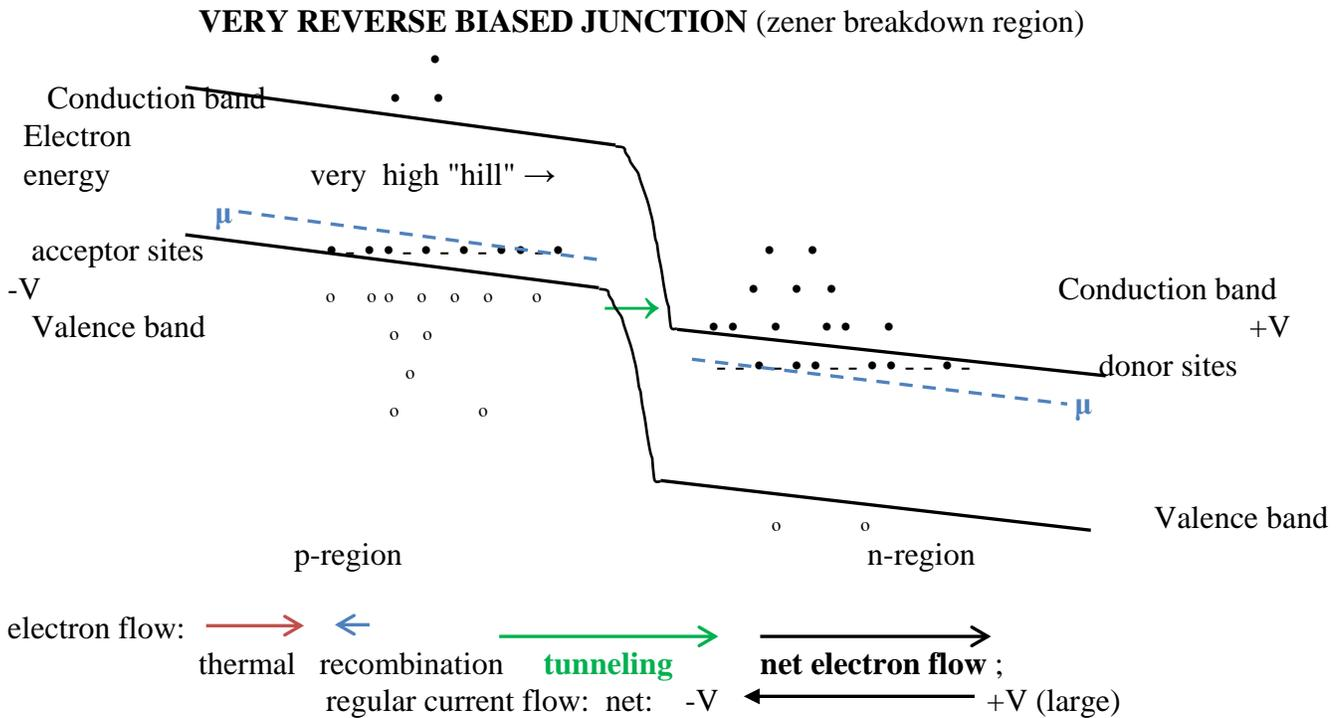
From the tunneling that occurs, the current going from the -V to the +V increases dramatically! To prevent damage, a current limiter is usually employed with zener diodes.
