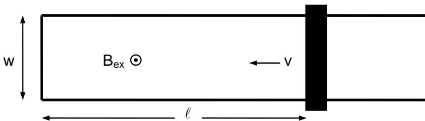
The conducting bar is moving at a speed of 12 m/s ( $v$ ) to the left across conducting rails that are 16 cm apart ( $w$ ). The present distance of the bar from the connected end of the rails is 40 cm ( $\ell$ ). The strength of the external magnetic field is a constant and uniform .37 T ( $B_{ex}$ ).
